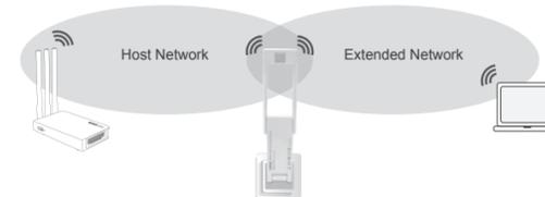
**2** In order to make full use of extender, please keep the antennas of the extender perpendicular to the horizontal plane. See below:
