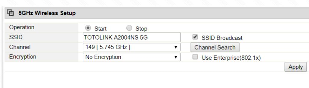
**Note:** You must select Start in the Operation bar firstly, after configuring the parameters, don't forget to click Apply.
