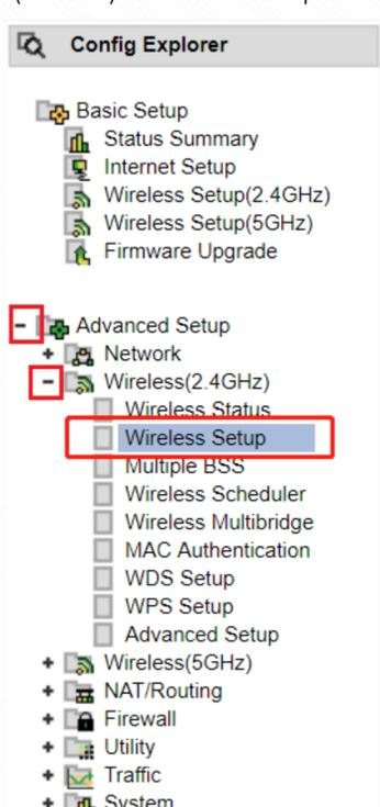
From the option, you can setup wireless parameters of 2.4GHz band
