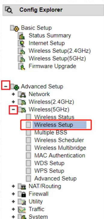
From the option, you can setup wireless parameters of 5GHz band
