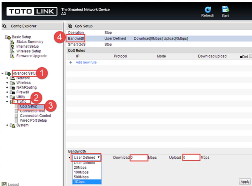
Or you can fill in **IP Address** and **Down** and **Up Speed** you want to restrain, then Click **Apply**.
